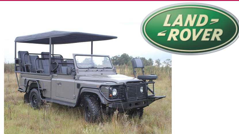
Prototype fully electric Land Rover Defender
